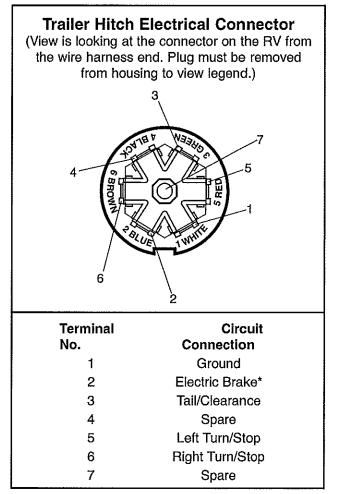
\*This circuit is provided to allow the use of a controller for electric brake actuation of a towed trailer or vehicle.
