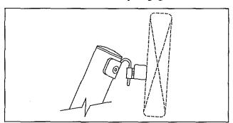
3. Ladder should be in an angled position to the floor, with both legs resting evenly on the floor, and both ladder hooks fully engaged.
