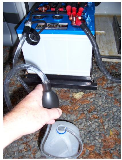
In asking around, we have found that many savvy owners, not only of motor coaches, but of all sorts of other equipment that depends upon wet cell batteries for power, use this clever system to maintain the proper level of electrolyte in their batteries.
