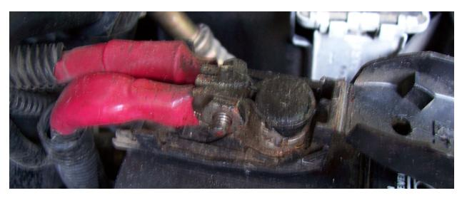
Because we were totally unaware that this connection was not tight, the chassis battery was discharged completely and repeatedly, quickly leading to its expensive demise.
