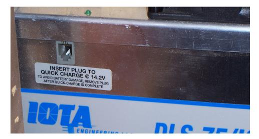
Needless to say, because of its inaccessible location and the fact that there was no information about it in our Owner's Manual, no one had ever removed it! No wonder we had boiled our batteries! I immediately removed the jumper plug, and we are happy to report that we have not boiled a battery since, and the water levels in the world's oceans has stopped going down since we are no longer consuming so much distilled water.
