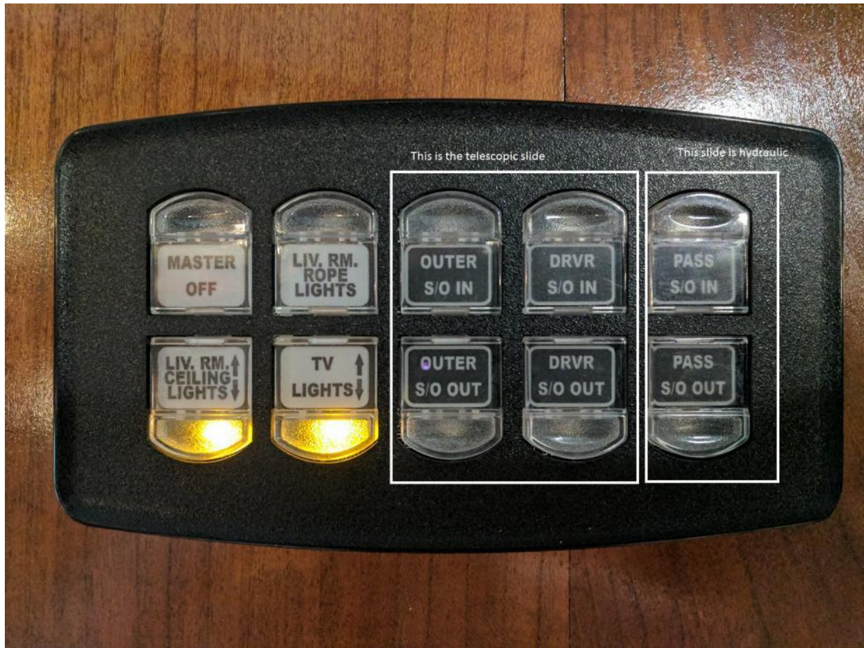
Control panel for telescoping slide room.
