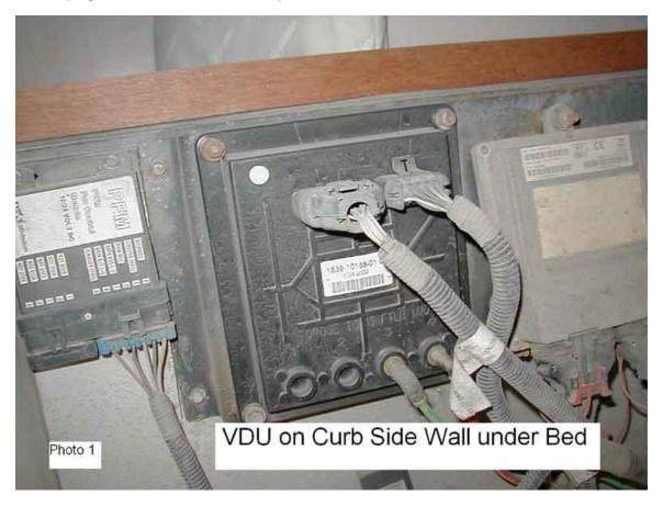
The full range of VDU problems indications is not known, but it is a fairly good bet that any false instrument indication may well be traceable to this unit. Some have reported various false indications which Freightliner dealers have resolved by replacing the VDU. On Jim Godward's and Jim Epting's units, the VDU caused false low air brake pressure warnings, including both the light and the gauge. It is only
