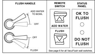
before another flush cycle can be initiated. A full holding tank will also prevent the toilet from flushing.
