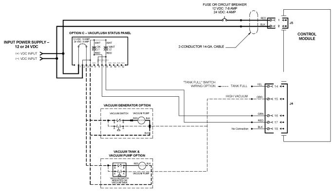
**IMPORTANT:** ORANGE WIRE ON PIN 15 OF CONTROL MODULE MUST BE CONNECTED TO THE "A" TERMINAL OF THE VACUUM SWITCH REGARDLESS OF WHICH VACUUM SOURCE IS USED.
