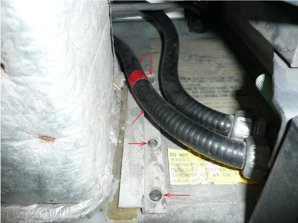
6. Remove (or loosen) the 2 screws if it is possible (if not too corroded). These sheet metal screws are going into heavy angle iron and can be difficult to remove. It may be possible to remove A/C unit without messing with this bracket. I was able to back out 3/8 inch & that allowed plenty of clearance.
