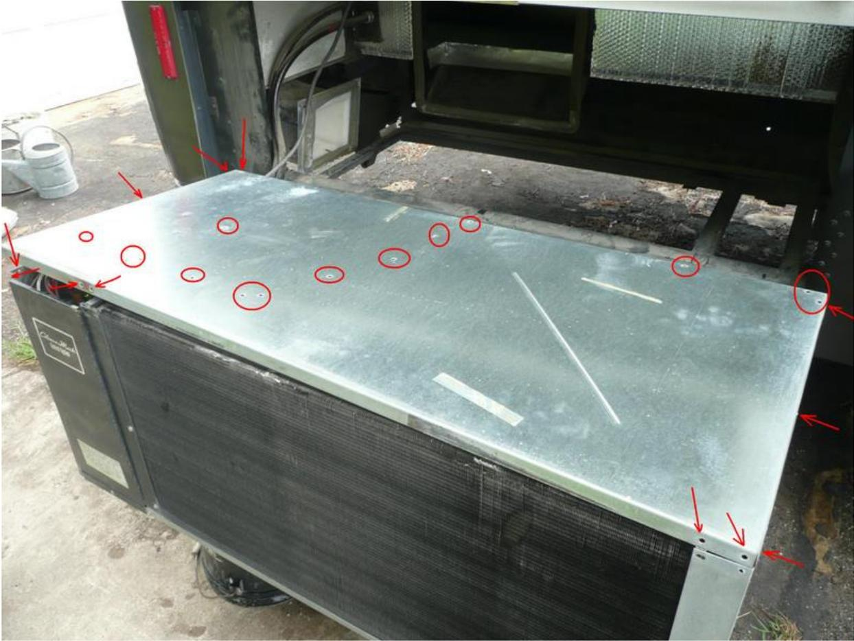
13. Remove these two additional screws to allow the condenser coil to be opened at the top if you need to pull the outdoor blower assy.
