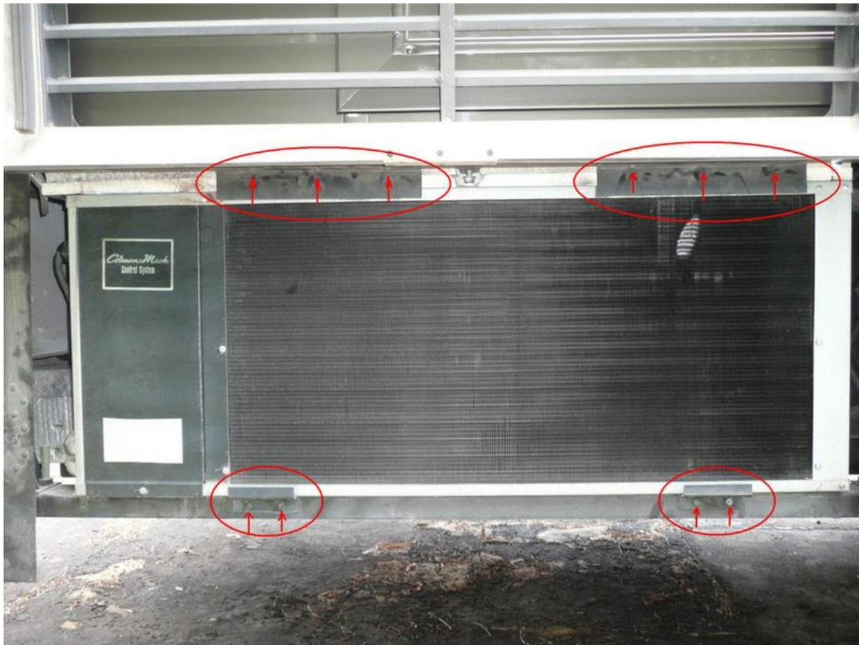
4. Remove 5 screws on left side of the cold air output duct. Good news is that there are no screws across the top!
