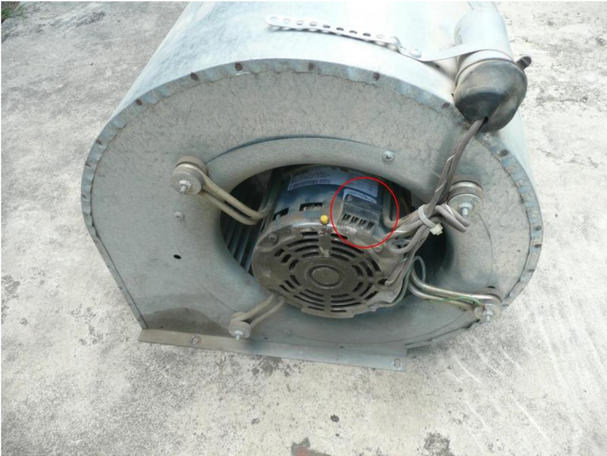
18. To replace the motor and/or squirrel cage, remove the 4 ea screw & nuts. Disconnect the two brown wires from the starting cap. Note the brown/white connects to the bottom spade lug (behind the rubber cover). Also note the motor bracket is not symmetrical & when re-assembling, make sure the wire connector is at the top.
