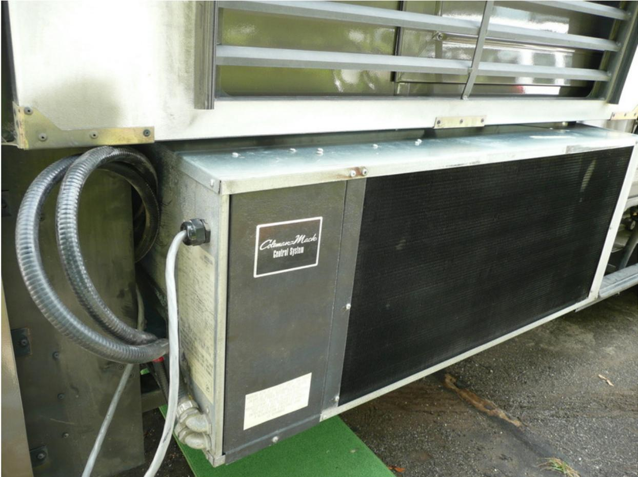
10. Support the unit off the ground to make it easy to carry, work on, and test while still keeping all the cables connected. I built a bench from two 5 gal buckets and two 2x6 planks. This was plenty strong and stable. Earlier in the campground I used the bench part of a picnic table. Leave open space under the Outdoor Blower screen so you can run the unit with the top panel off and test everything before closing up.
