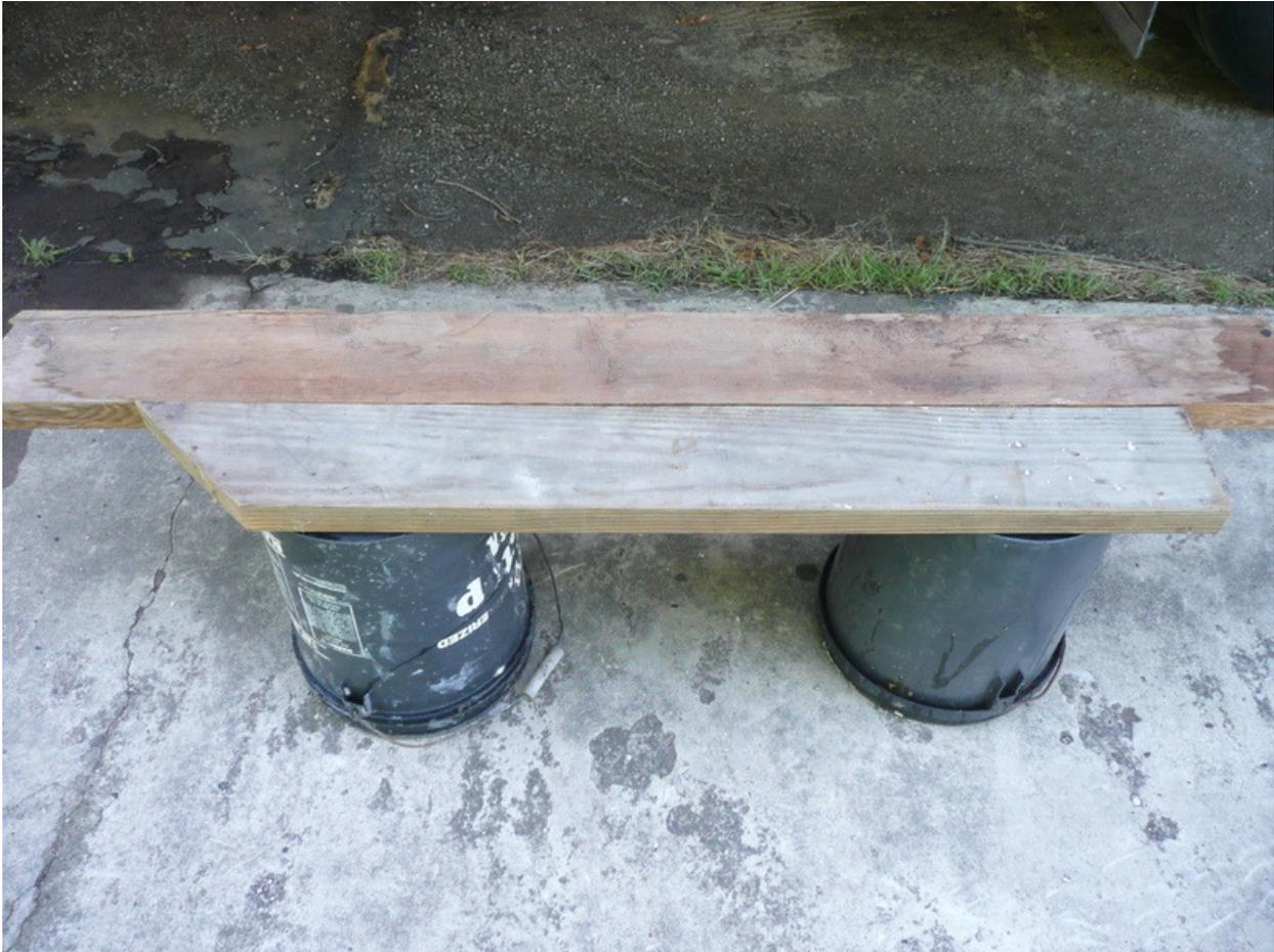
11. Use two people to pull the unit out and sit on support bench. The left side has a nice hand hold using the cold air duct opening. The right side has the two compressors and is somewhat heavier so the stronger guy should take that end. I'm no weight lifter and didn't have any problem getting the unit in/out two times with no muscle or back strain. Once you start pulling it out the two top styrofoam pieces will drop down.
