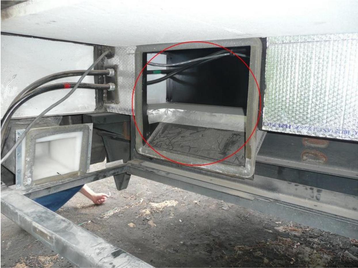
23. Reinstall the top cover using the approx 28 screws. Use a pointy object like an awl to align some of the holes in the middle of the top panel. Put the two screws back in front of the right side panel. Slide the entire unit back in coach. Once the unit is partially in, then feed the power cables up and over the duct. Re-install the four brackets.
