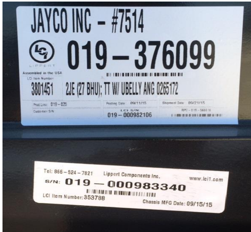
Chassis Tag: Large Sticker (top pic) is located on the curb side front of I-beam for both Travel Trailers and Fifth Wheels.
