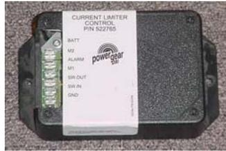
The two-stage S/O control can be adjusted to three settings – Low, Medium and High. For optimum slide-out operation, the control should be set at the High setting.
