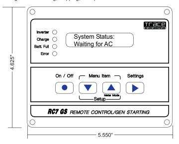
Install the RC7GS as described earlier. Be sure the inverter/charger is disconnected from the AC power source and the On/Off switch on the inverter is in the Off position. Plug-in the RC7GS and turn the On/Off switch on the face of the inverter to the On position.
